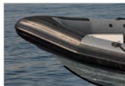
Reinforced tube at bow
