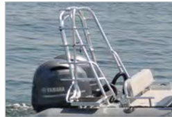
Antenna arch with dive ladder
