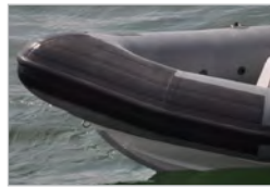
Reinforced tube at bow
