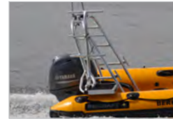
Antenna arch with dive ladder
